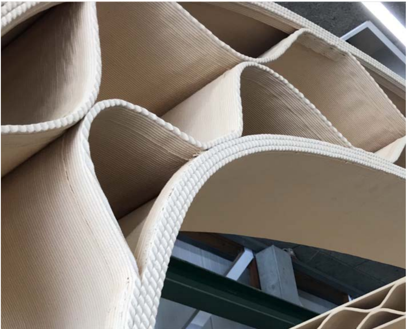
Segmented print concepts – load bearing shells and full frame structures.
