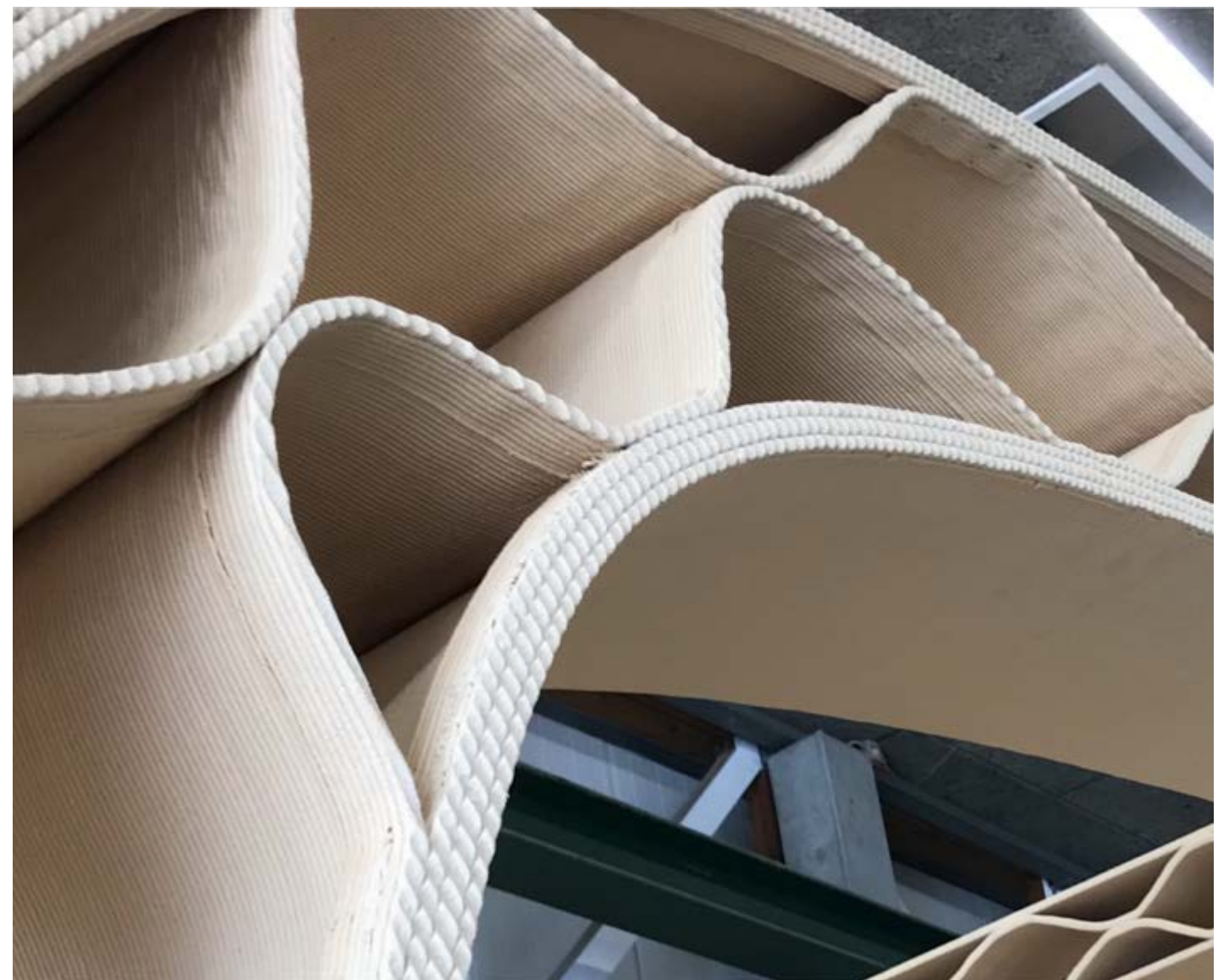
Segmented print concepts – load bearing shells and full frame structures.
