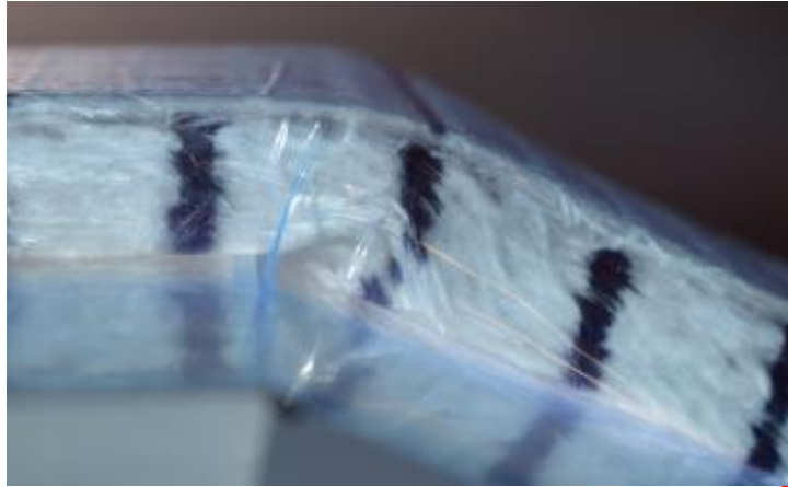
Large wrinkle with delamination
