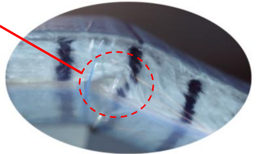
Wrinkles are associated with high curvatures!
