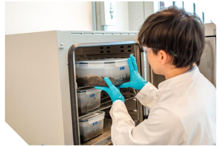
ISO 20200 laboratory scale disintegration
